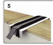
Capping profiles consisting of colour coated or pre-weathered finishes, place a small 40mm - 45mm wide strip of the same material in the centre of the joint.
