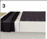
Lay ISO-Mat Metal separating membrane between the connectors, over the fixing strips. Hook the capping profile onto the fixing strip on one side.
